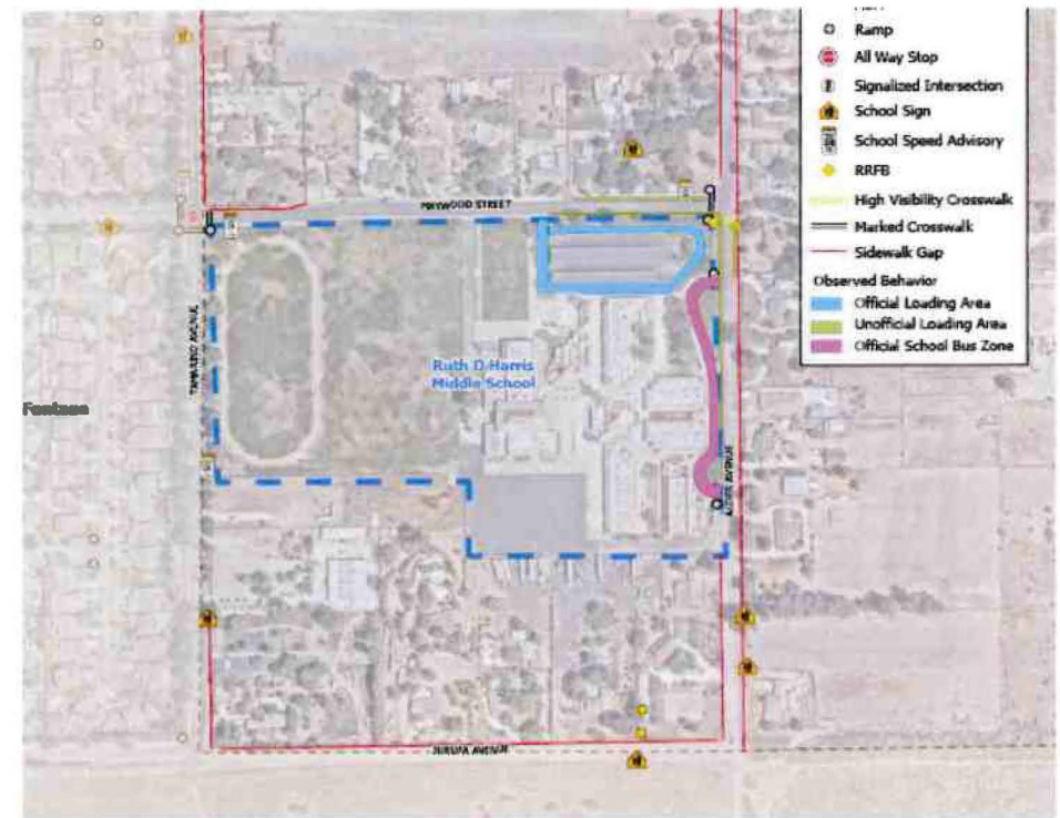
Figure 4.4.15 Existing Pick-Up and Drop-Off Vehicle Behavior
