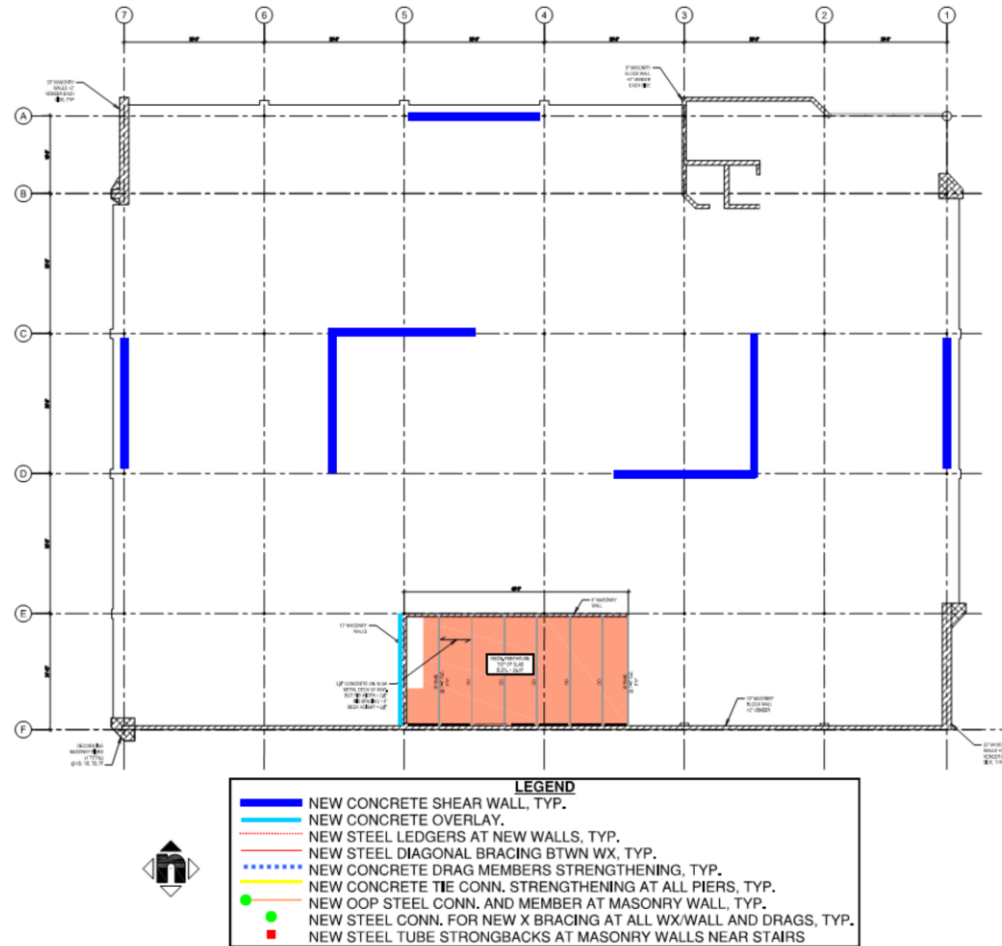
Figure 5-5: Option No. 1 – Mezzanine Level Strengthening
