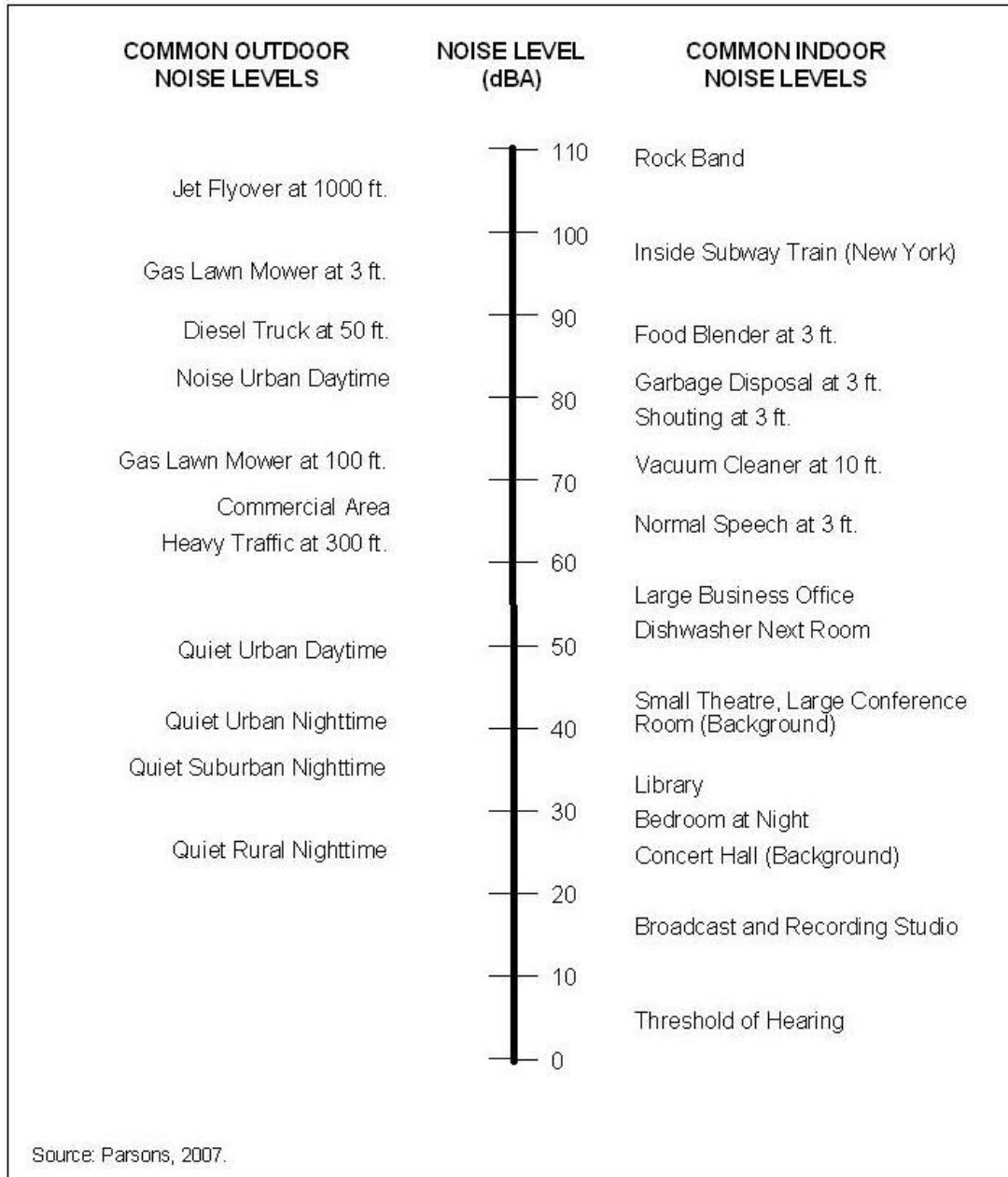
Figure 2.12-1 Typical Sound Levels from Indoor and Outdoor Noise Sources
