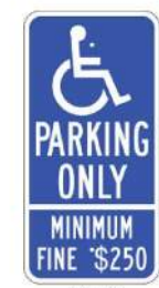
R99C PER CBC 2022 SECTION 11B-502.6 & 11B-502.6.2 NOTE: NON-VAN ACCESSIBLE PARKING STALLS ONLY
