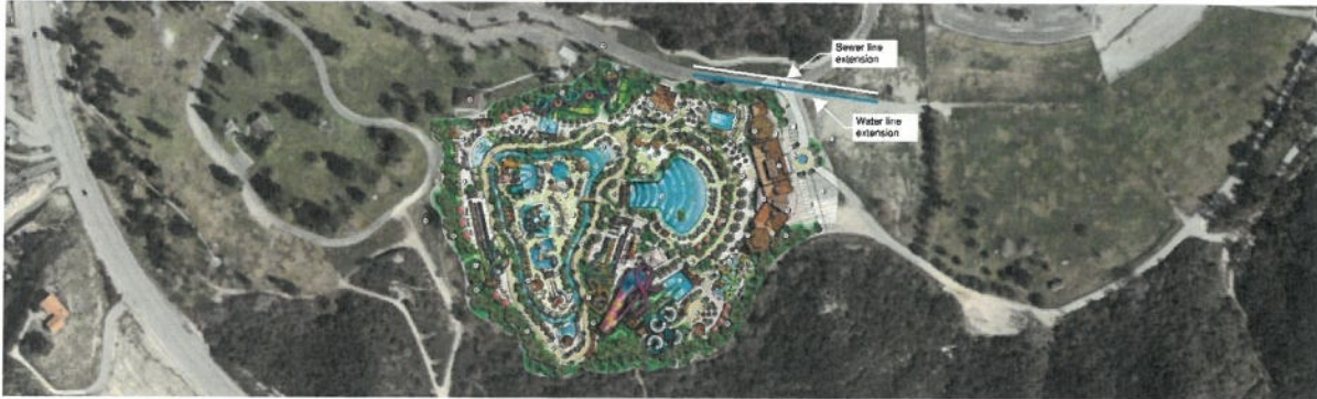
Figure 51 Adventure Park water and sewer extension
