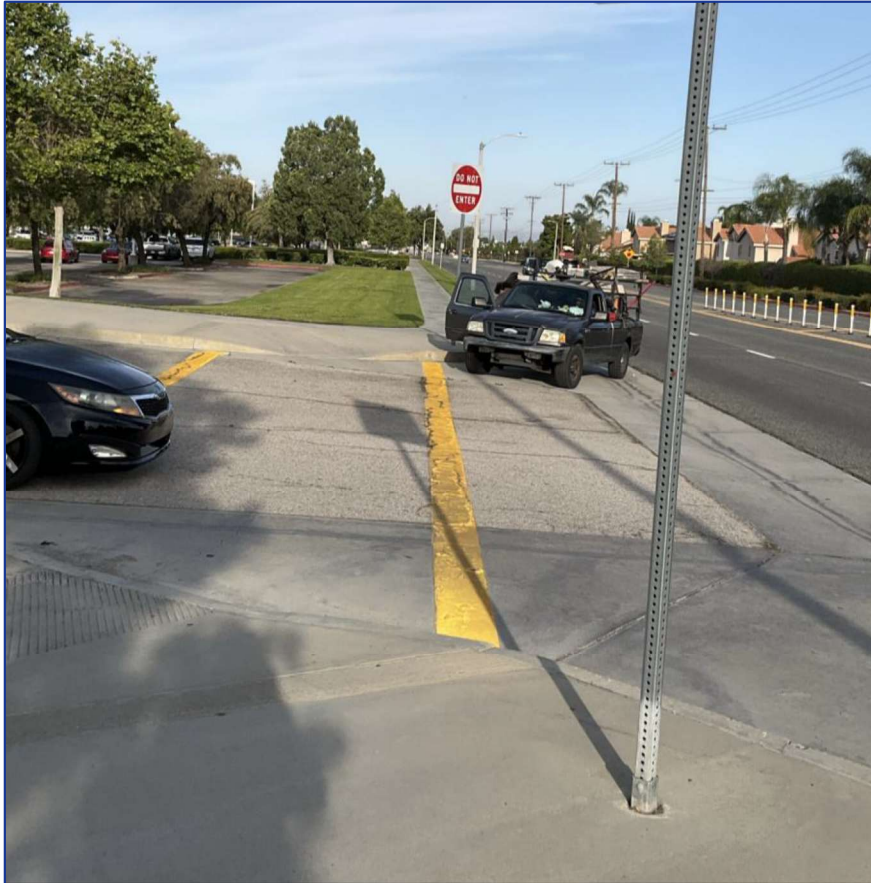
REVHS campus driveway along Colton Avenue, illustrating vehicle encroachment, turning conflicts, and unclear pedestrian circulation at a high-use student access point.
