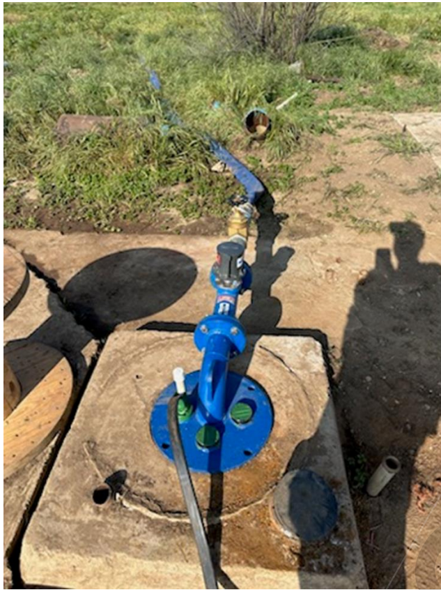
Figure 5a: Test Pump, meter, and discharge hose set for pumping test.
