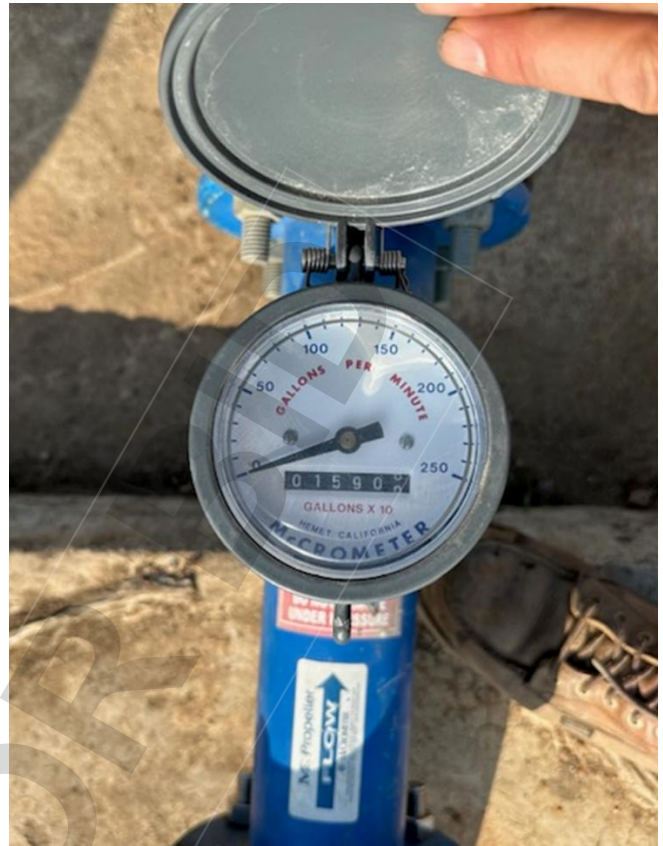
Figure 5b: Meter reads 15900 at start of Pumping test, estimate flow from testing ~180,000 gallons.
