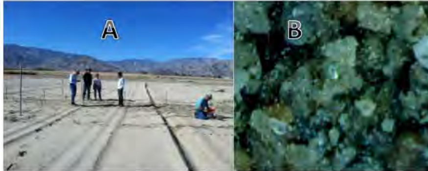
Figure 10: The CVARS solar-simulation site (A) and a hi-resolution in situ AMR image of the soil (3.01mm X 2.26mm, 100x image) showing soil particles.
