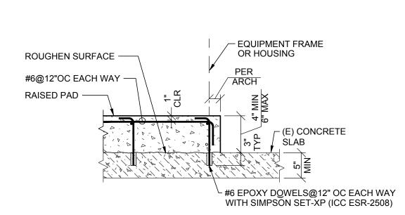
1. FOR SIZE, AND LOCATION OF RAISED PADS SEE ELECTRICAL DRAWINGS UNO. EXTEND PAD MIN 18" PAST GENERATOR ON ALL SIDES. 2. GENERATOR ANCHORAGE SHALL BE MIN (4) 1/2" DIA HILTI KB-TZ ANCHORS (ICC ESR-1917) W/ MIN 2" EMBEDMENT.
