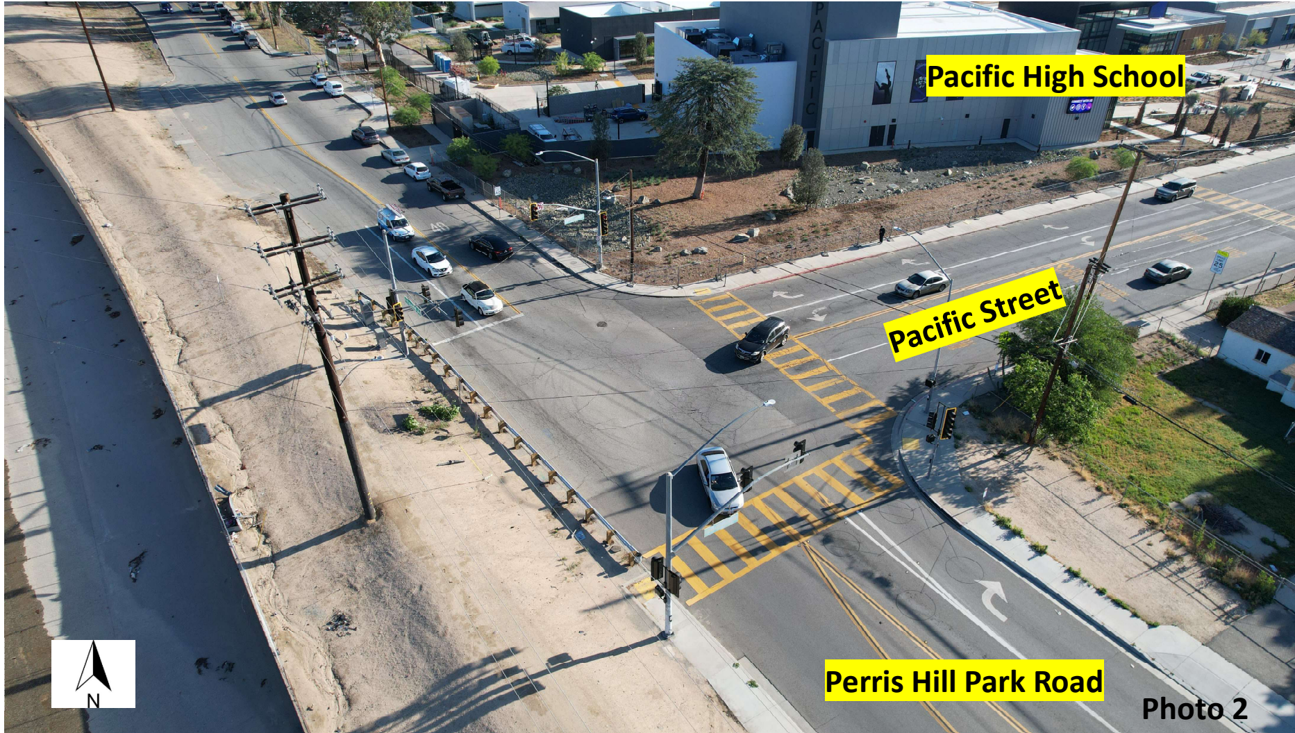
Photo 2 shows the three-way intersection at Pacific Street and Perris Hill Park Road looking north. There are no bike lanes, and no sidewalks on the west side of Perris Hill Park Road, the route from Pacific High School to the San Bernardino YMCA .7-miles north.
