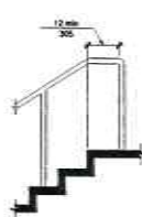
FIGURE 11B-505.10.2 TOP HANDRAIL EXTENSION AT STAIRS
