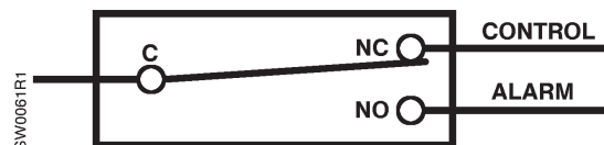
Figure 7. Auto Reset Switches to Prove Excessive Airflow or Pressure.
