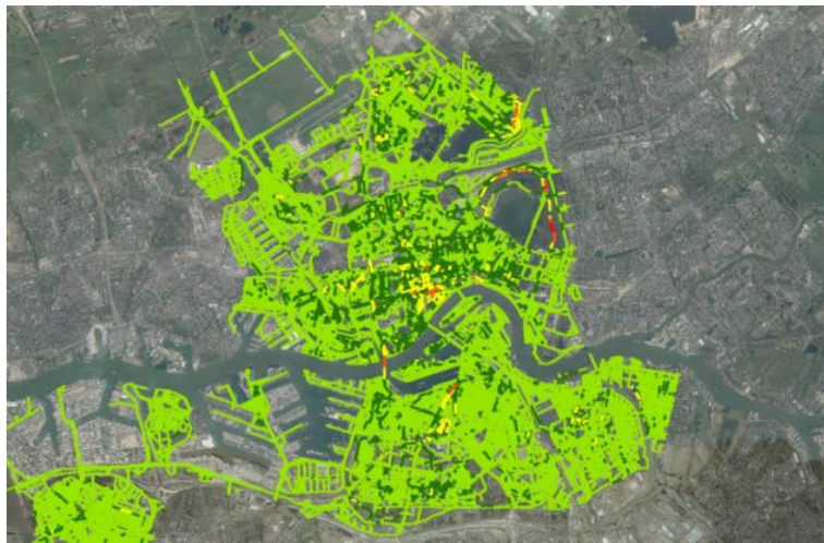
Figure 1: Green shows high positional accuracy, red is poor positional accuracy due to minimal GPS/IMU signal under urban canyons and dense vegetation.
